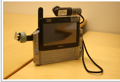
Fig. 2. The display devices. On the left, the head-mounted display (HMD), a wearable virtual see-through near-to-eye display with an integrated gaze tracker. On the right, an ultra-mobile PC (UMPC), a handheld computer with a virtual see-through display.
