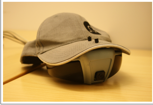
Fig. 2. The display devices. On the left, the head-mounted display (HMD), a wearable virtual see-through near-to-eye display with an integrated gaze tracker. On the right, an ultra-mobile PC (UMPC), a handheld computer with a virtual see-through display.
