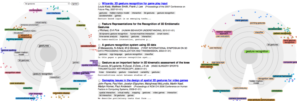
Figure 1: Left: IntentRadar interface. The system uses a radar metaphor. The current intent estimate for which the results on the right-side list are retrieved, is visualized as keywords on a radar screen (inner dark grey area). Predicted alternative intents, that help users explore their information need, are shown as keywords in the outer (light gray) area, organized as directions on the radar. In both areas, radius corresponds to relevance of keywords (closer to center = more relevant) and angular distance between keywords corresponds to directions of search (technically: similarity of how keyword relevance would be affected by potential feedbacks). The keywords can be enlarged with a fisheye lens that follows the mouse cursor. The user can give feedback by dragging keywords closer to (or away from) the center of the radar. Right: after feedback. The user increased relevance of "gesture recognition" by dragging it to the center of the radar. The system computed and visualized new estimated relevant intents, such as "pointing gestures", "recognition rates", and "hidden Markov models". Documents are retrieved for the new intent estimate. The user can continue exploring the new intents.
