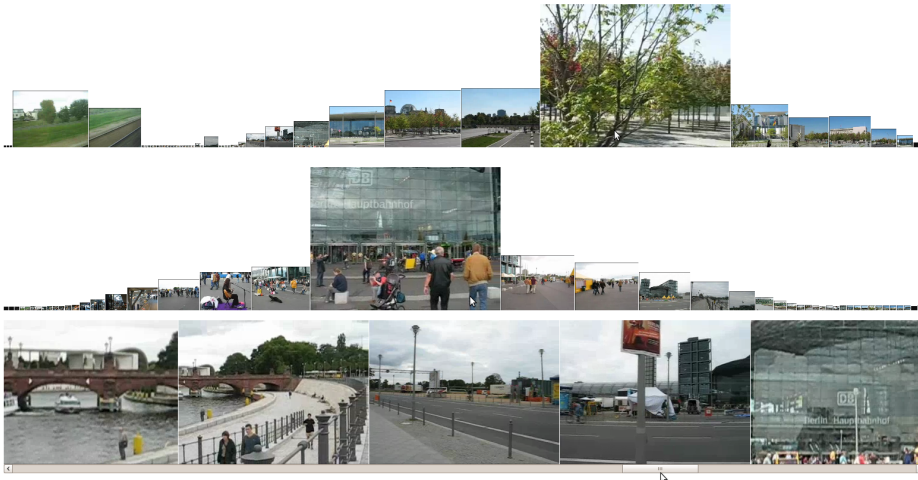
Fig. 1. The three interface variants from the experiments. From top to bottom: our new proactive interface where image sizes are proportional to the estimated relevance, zooming interface that magnifies the image on which the cursor is located and its neighborhood, and a scrollable simple timeline. The images are snapshots from a Creative Commons licensed movie by Adam Wojtanek.
