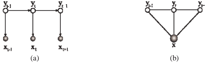
Figure 1: Dynamic representation of HMM (a) and CRF (b) as graphical models, where grey nodes represent observed variables.
