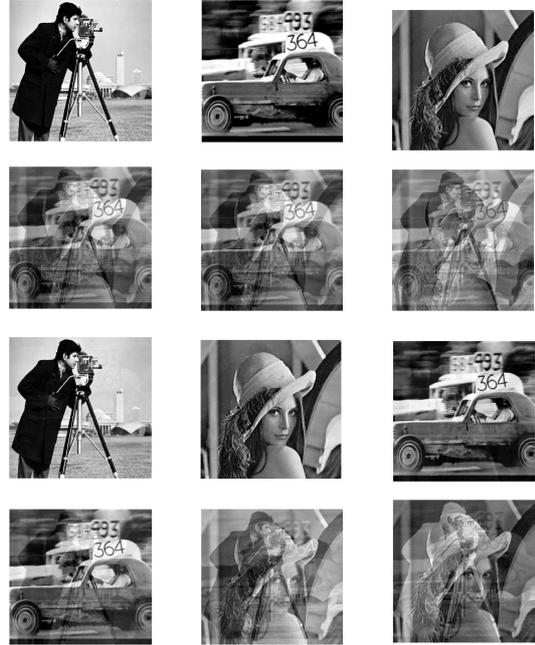
Figure(7): ‘ICA with OS’ and ‘INFOMAX’ for an arbitrary mixture of three images. Top: Original images; Second row: mixtures, Third row: Separated images though ICA with OS (-11 dB); Four row: Estimated images though INFOMAX (-2 dB).
