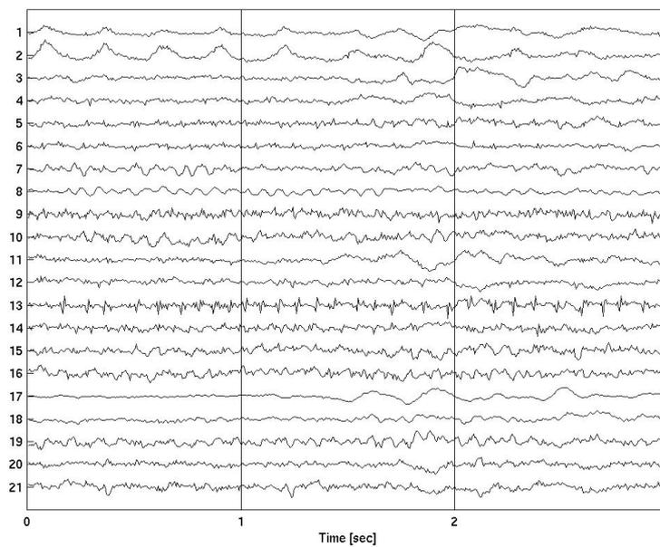
Figure 6. ICA components obtained from EEG sensors
