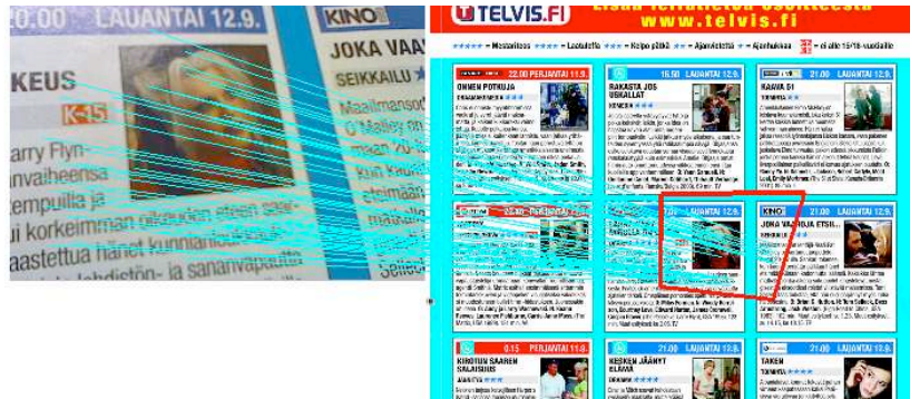
Figure 7.3: An example of matching an image captured with a mobile phone and the corresponding magazine page.
