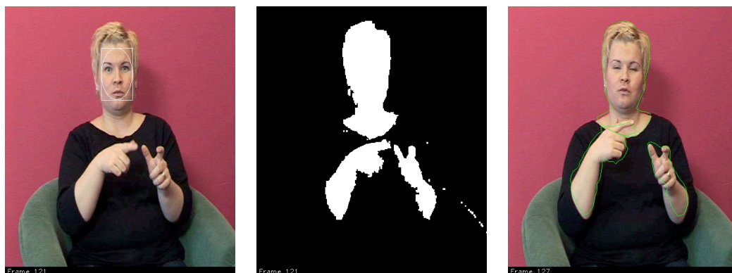
Figure 7.2: Example frames from the sign language video material. From left to right: Face detection, skin-color filtering, active shape models of skin regions.
